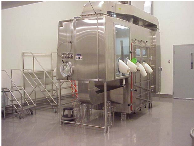
Horizontal Uni-directional Flow Combo Isolator. Used for drum lid removal, cone placement and drum separation.
