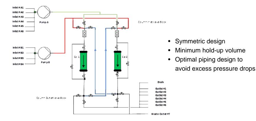
More robust operations with less risks due simplicity in process and equipment. Fewer hardware components (pumps, valves, piping)  $\rightarrow$  less risk for breakdown Lower CapEx investment and footprint !
