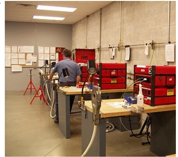
Figure 4. Arc Machines Model 207 power supply Model 8 weld heads used in the manufacture of bioreactors and fermentors. Photo courtesy of Sartorius BBI Systems, Inc & Arc Machines, Inc.
